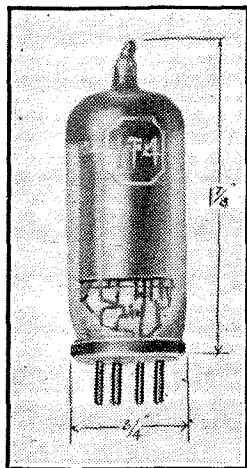
Valves used in American personal receivers have 1.4 volt filaments taking 50 or 100 mA. Separate bases are dispensed with and extensions of the electrode supports serve as base pins.
